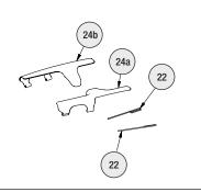
Flip covers (item 23 or 24a and 24b) are not required if the unit is equipped with a bowl and cover. These flip covers can be removed and discarded by installer.
