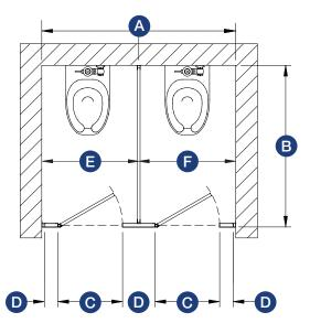
Refers to a compartment or compartments located between two walls. Shown below as one 60" (1524 mm) compartment and two standard 36" (914 mm) compartments.
