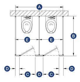
Refers to layouts where the compartments will be located without being affixed to lateral walls. Shown below as one 48" (1219 mm) compartment and two standard 36" (914 mm) compartments.
