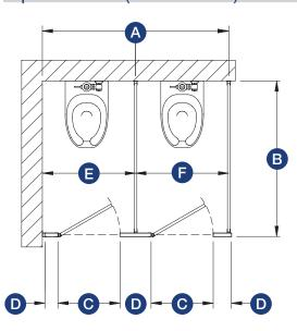
Refers to a compartment or compartments that will be affixed laterally to only one wall. Shown below as one 60" (1524 mm) compartment and two standard 36" (914 mm) compartments.
